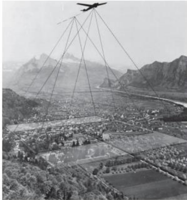
Figure 2.2 Acquisition of successive photographs yielding a stereopair.
